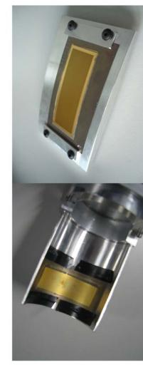
Gratings made by KIT on flexible titanium substrates.
