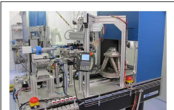
Figure 4: The assembly of the mirror plates into stacks is performed by automatic stacking robots, remotely controlled by operators. The time required to mount a mirror plate is only a few minutes, and the figure of each plate is inspected after mounting, using fringe reflection metrology (located in the blue box on the right). The surfaces of the mirror plates are so smooth, that they are fixed to each other by hydrophilic bonding. No glue is used to assemble the mirror stacks.
