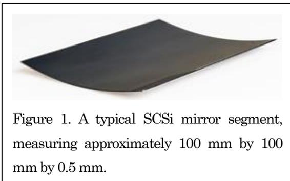
The dimensions of the basic mirror element are determined by a combination of several factors, including dimensions of easily available and affordable single crystal silicon blocks, semiconductor industry processing equipment, gravity distortion when the mirror segment is kinematically supported at four optimal locations, and the fact that shorter axial lengths lead to better off-axis PSF.
